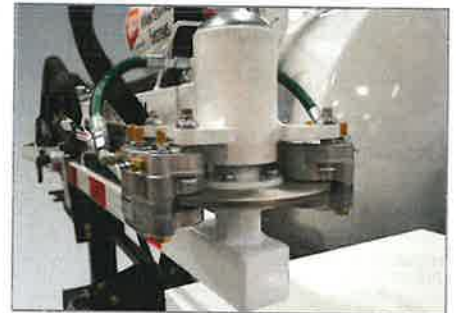
ERV-750 uses unique disk brake system for rigidity, and hydraulic sensors for true hands-free operation
