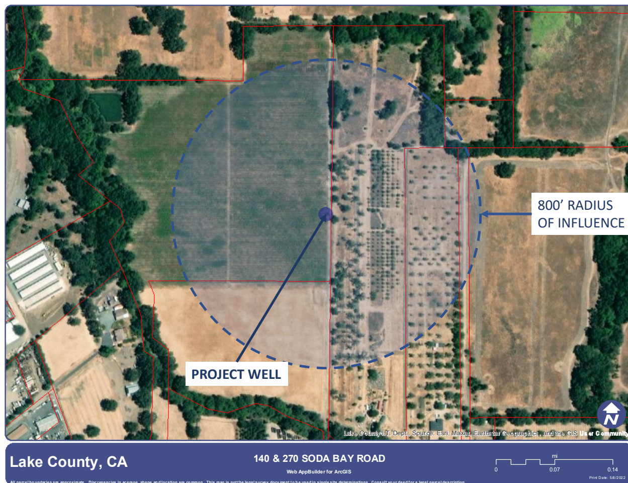
Figure 2 – Zone of Pumping Influence Diagram
